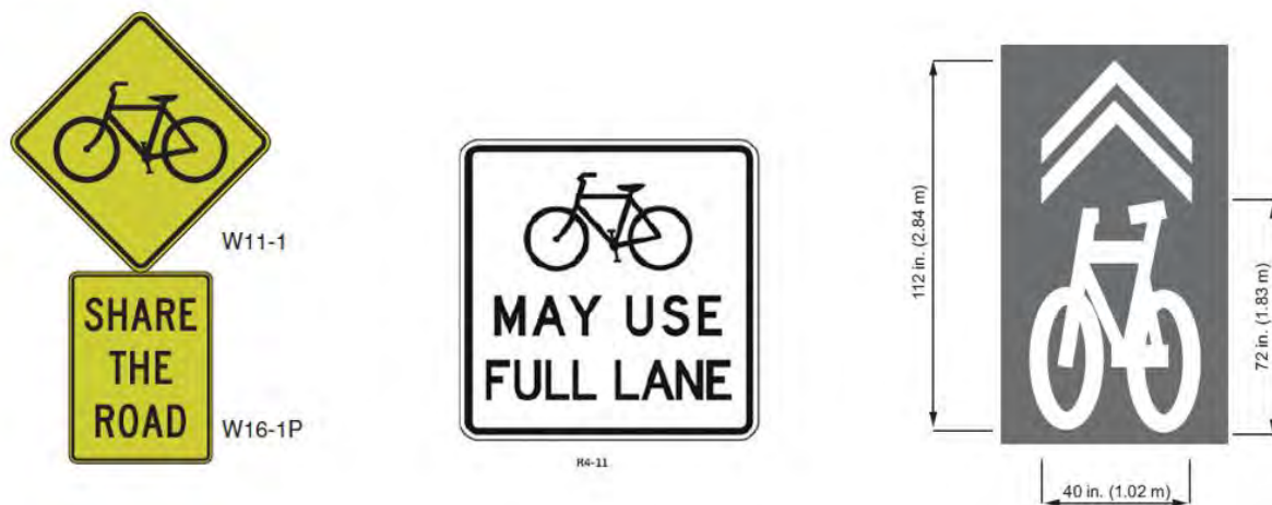
Figure 57. Example of Bicycle-Specific Signs and Pavement Markings [A.1, A.25]
