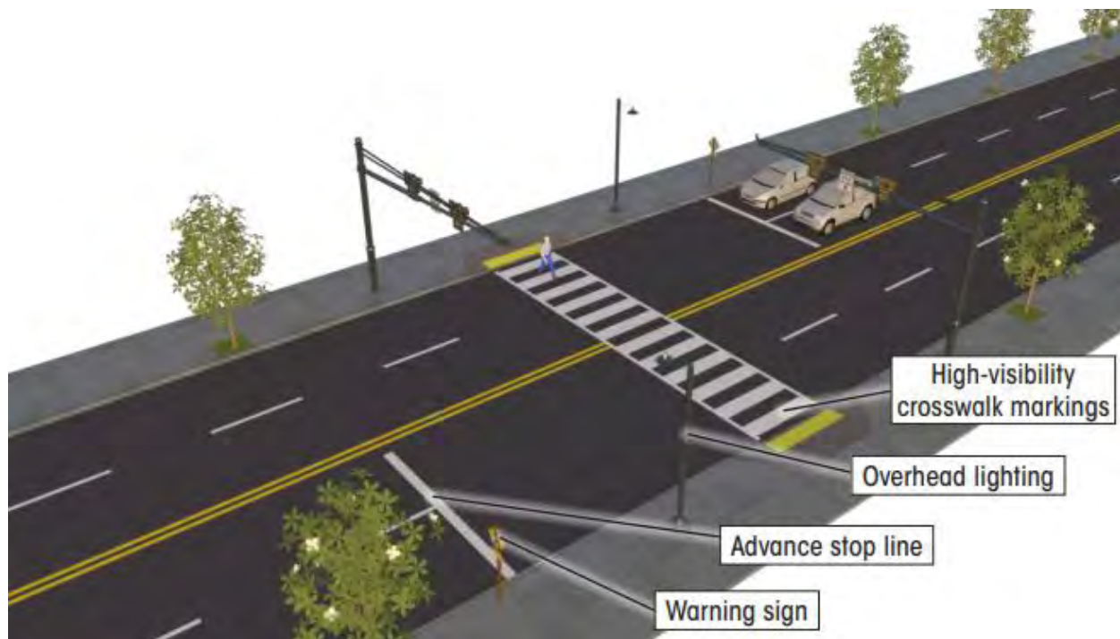
Figure 24. Example of a Pedestrian Hybrid Beacon [A.144]
