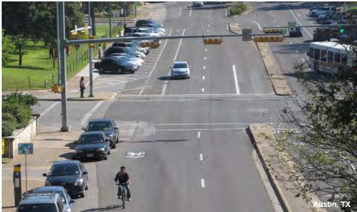
Figure 58. Example of Shared Lane Markings in Austin, Texas [A.12]
