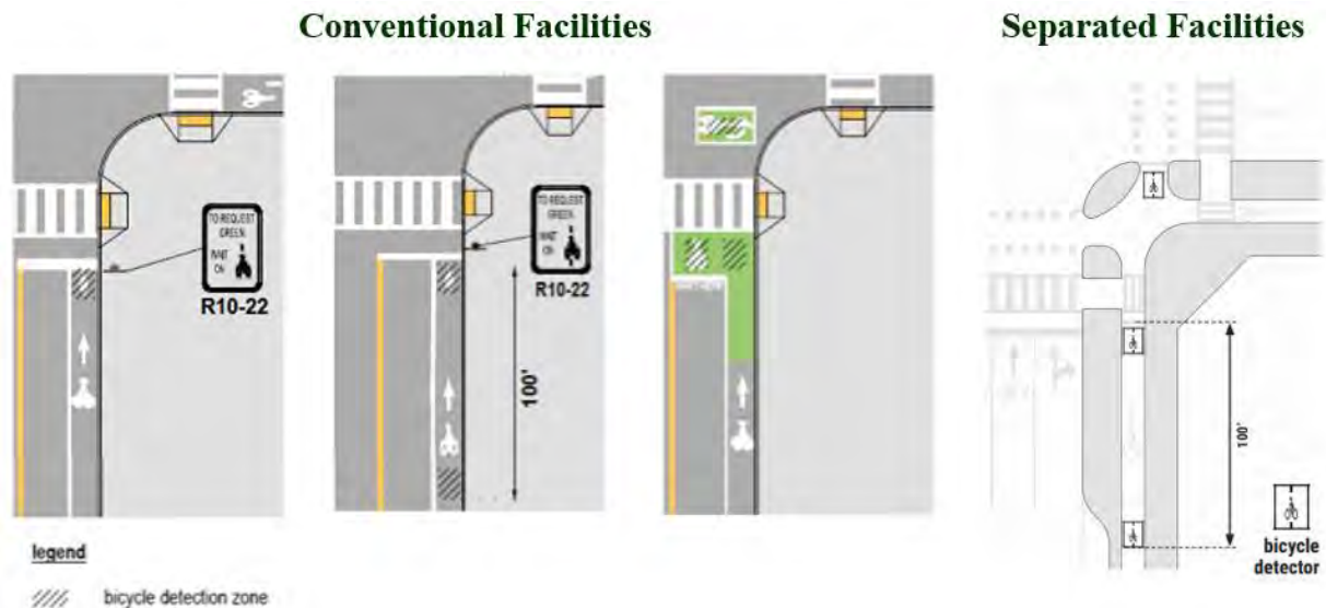
Figure 8. Bicycle Detection Zones at Conventional [62] and Separated Facilities [19]
