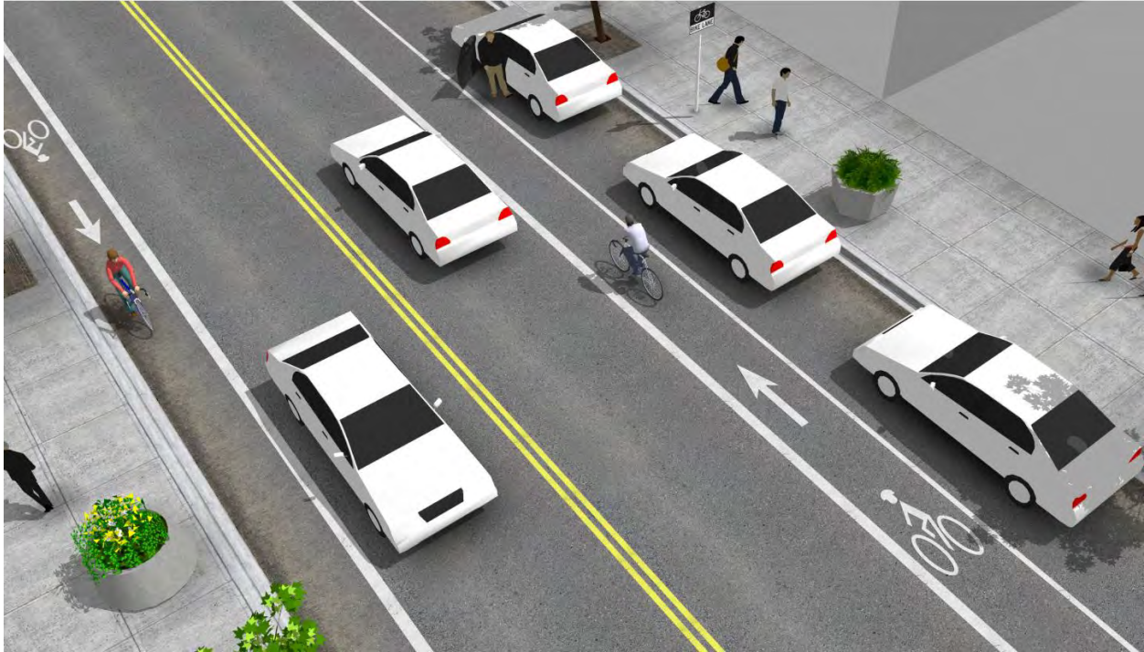
Figure 61. Conceptual Drawing of Conventional Bicycle Lane [A.12]
