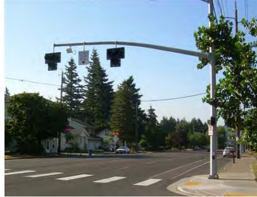
Figure 26. Example of Pedestrian Hybrid Beacon in Portland, Oregon [A.10]
