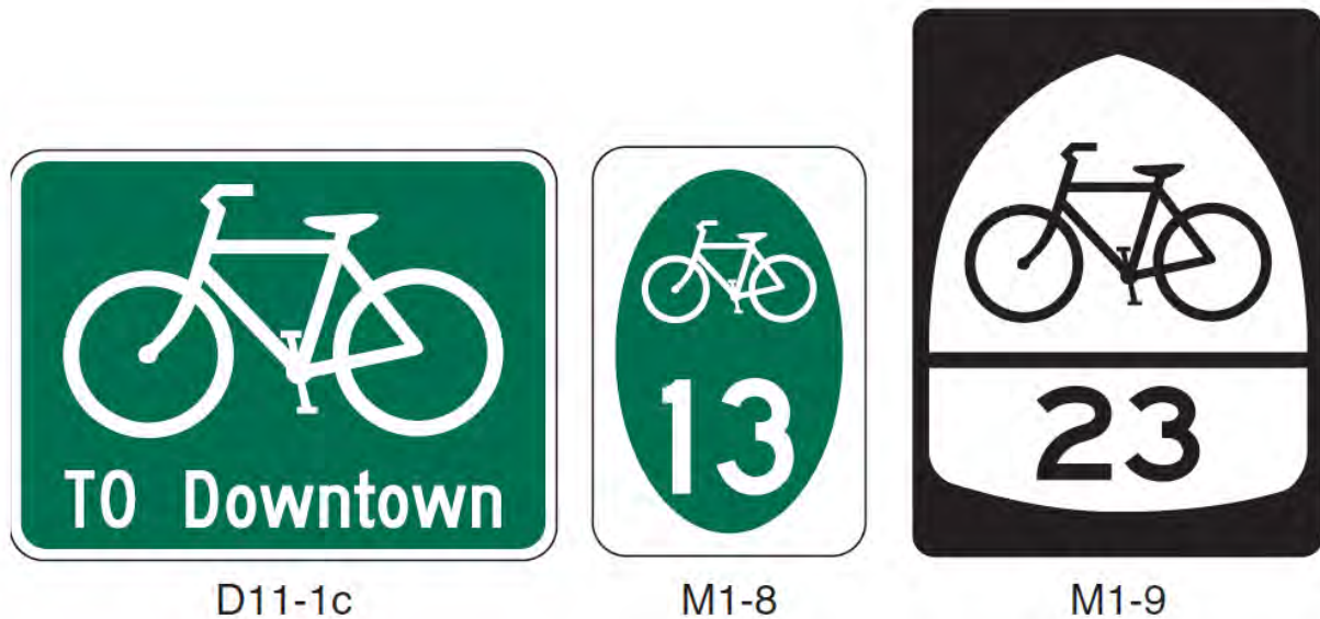
Figure 56. Typical Bicycle Wayfinding Signs [A.1, A.25]
