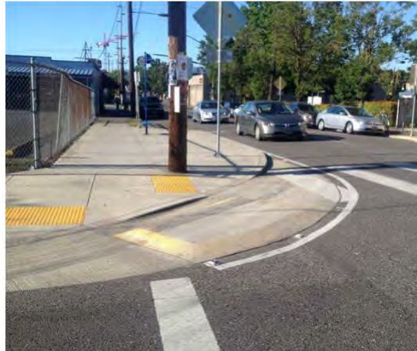
Figure 10. Mountable Truck Aprons Case Study Example from Portland, OR [A.10]
