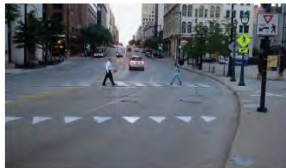
Figure 18. Example of Advanced STOP (left) and YIELD (right) Markings and Signs [A.150]
