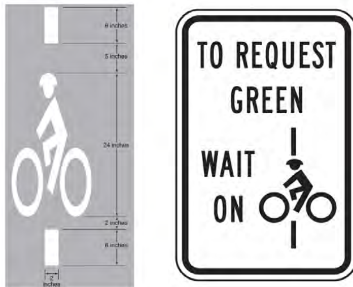
Figure 5. Bicycle Detector Pavement Marking (Figure 9C-7) and R10-22 Sign [4]
