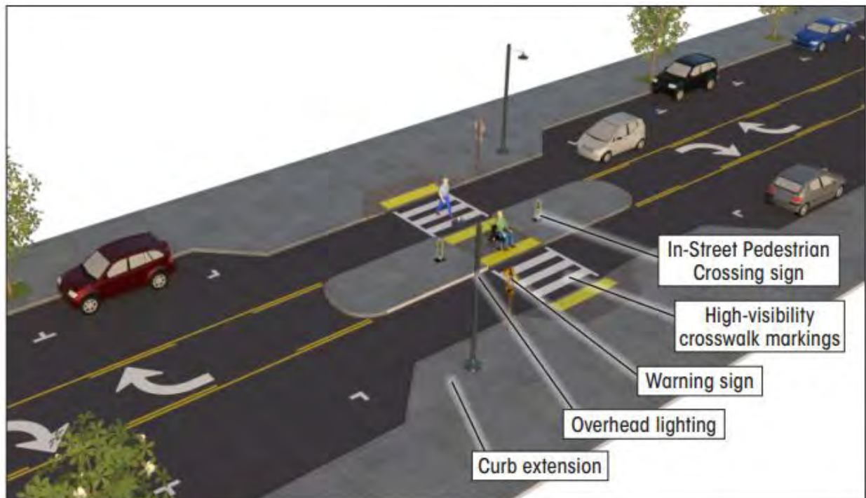
Figure 29. Example of Pedestrian Refuge Island [A.144]
