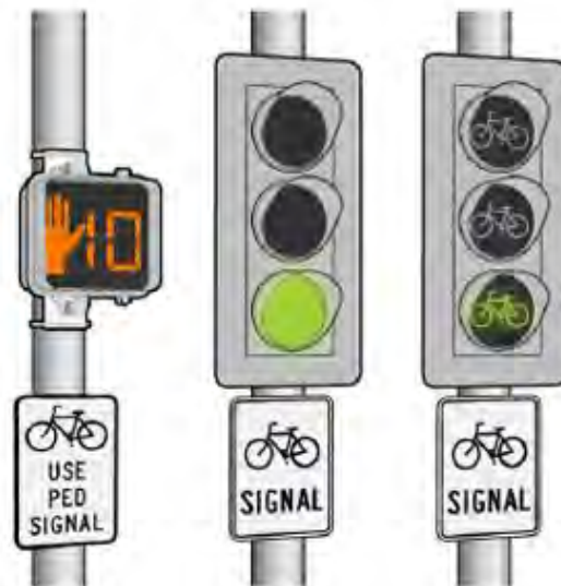
Figure 1. Options to Provide Signal Indications to Bicyclists, including Bicycle Signal Heads or Faces [15]
