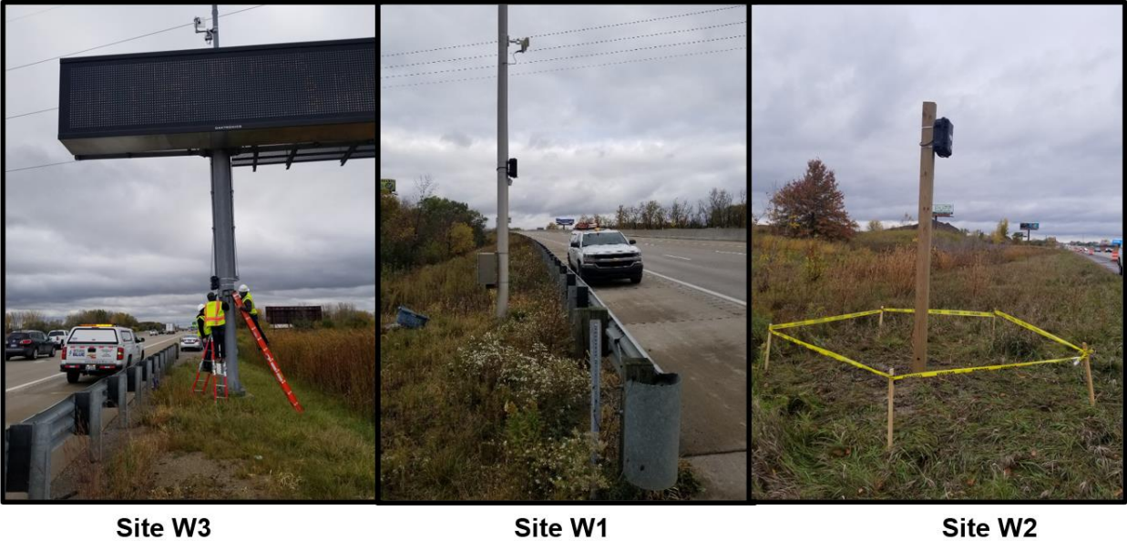
Figure 5.17. Examples of sensor mounting mechanisms
