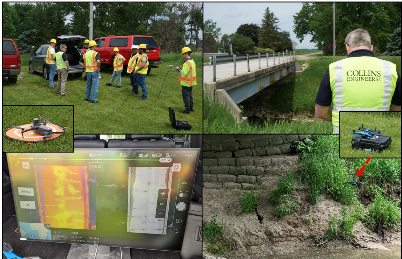
Figure 3.2.35: Left Panels: Live field demonstration of the dual optical thermal DJI Mavic 2 Enterprise Advanced at N Beyer Rd Bridge. Right Panels: Live demonstration by Collins Engineers' Barritt Lovelace of the Skydio 2 performing an autonomous survey (including bridge substructure) of the N Beyer Rd Bridge over Cheboyganing Creek.
