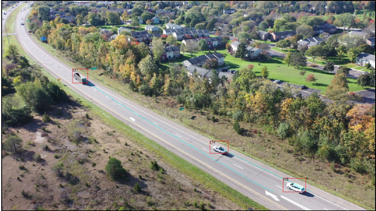
Figure 3.1.16: Automatic vehicle detection and tracking at US23/M14 weaving area.
