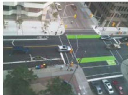
Traffic signal with pedestrian countdown signal (Chicago Metropolitan Agency for Planning n.d.) + Two stage turn ques boxes (National Association of City Transportation Officials 2012)
