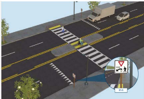
Advance yield here to pedestrian sign and yield line (Federal Highway Administration 2020b)
