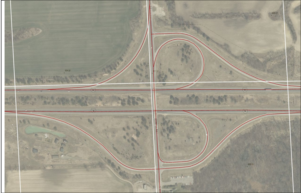
Figure 10. Some common reference GIS datasets include PLSS, road layers and orthoimagery. This example shows the differences in accuracy between the PLSS polygons (white outlines), the roads (red lines) and orthoimagery (MiSAIL Michigan Imagery Public image service). While none of these layers approaches the accuracy of surveyed points, the orthoimagery is likely the most accurate of the three. It is notable that the current PLSS data does not seem to match well at all. The reason for this is that it is not based upon recent survey data from the statewide re-monumentation effort. As this effort is completed, it is likely that the PLSS data layer will be adjusted to match the new surveyed points. Until then, the dataset Public Land Survey Corners and Remonumentations available from the Michigan GIS Open Data portal, could be used, though this dataset is incomplete.
