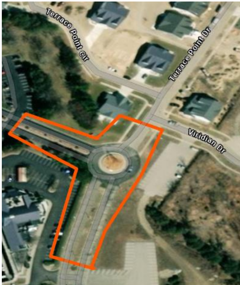
Figure 19 Example of Roundabout Adjacent to Another Intersection
