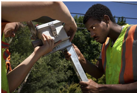
Figure 3. Mitchell Wojtowicz and Kenneth Ferrell deploying an Open-Storm Sensor
