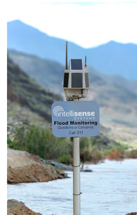
Figure SEQ Figure \* ARABIC 11: AWARE Flood System Source: Intellisense
