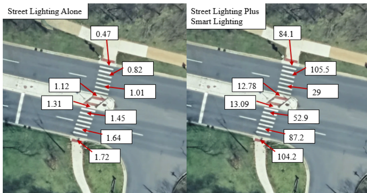
Figure 4-6. Lighting levels at each location in crosswalk with street light alone (left frame) and Street light plus smart lighting (right frame).
