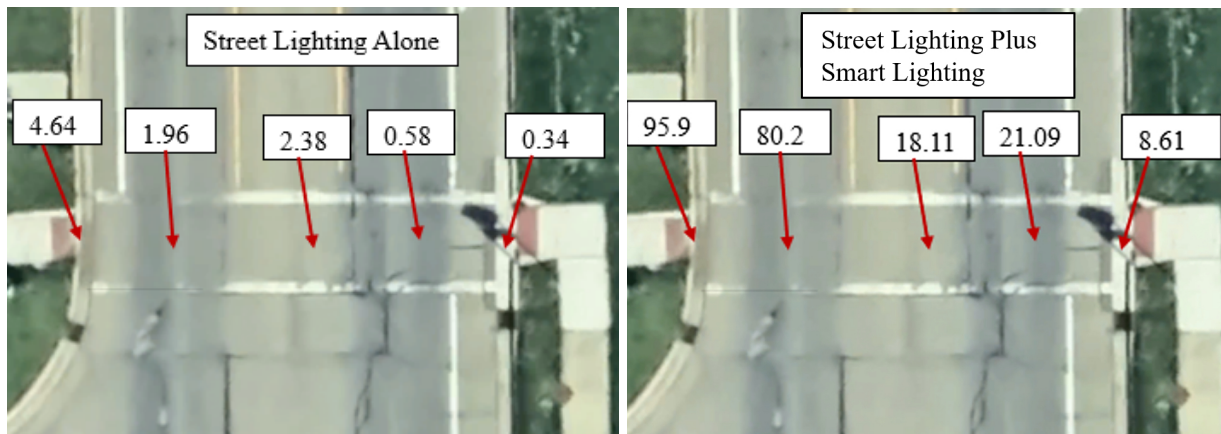
Figure 4-12. Lighting levels at each location in crosswalk with street light alone (left frame) and Street light plus smart lighting (right frame) at Oakland Dr. and Edgewood Drive.
