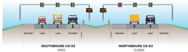
FIGURE A-4. EXAMPLE OF AN ATM "FLEX ROUTE" SYSTEM
