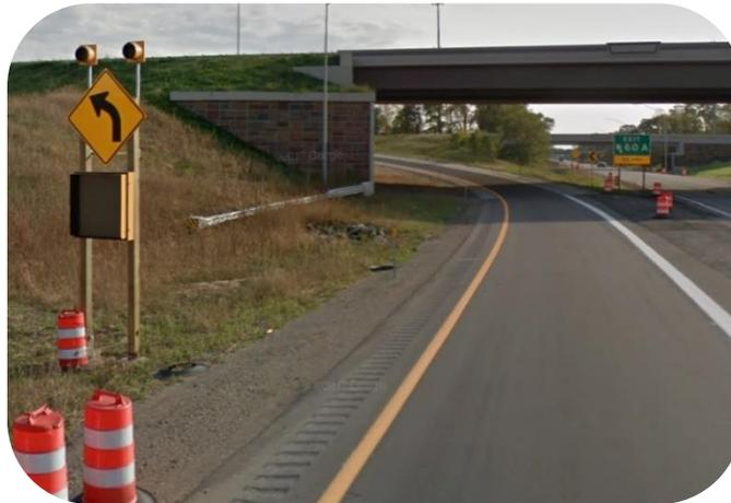
FIGURE A-11. EXAMPLE OF A CURVE SPEED WARNING SIGN
