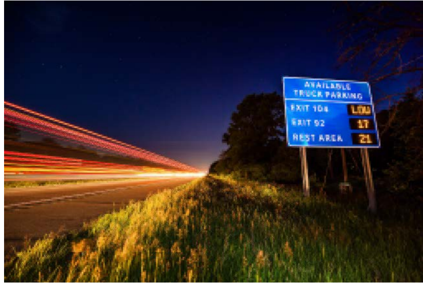
Figure 33: Dynamic sign consisting of three lines and six bits of information
