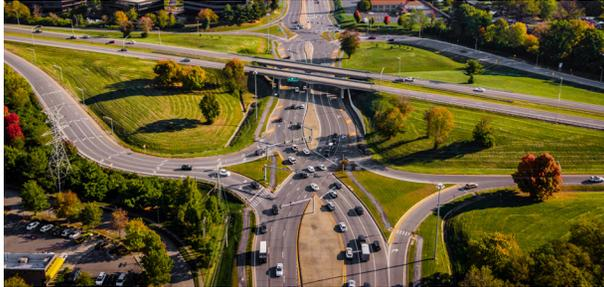
A Diverging Diamond Interchange (DDI) is an alternative interchange that improves safety, increases traffic flow, and reduces construction cost.
