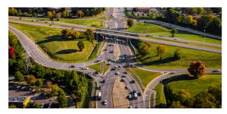
A Diverging Diamond Interchange (DDI) is an alternative interchange that improves safety, increases traffic flow, and reduces construction cost.
