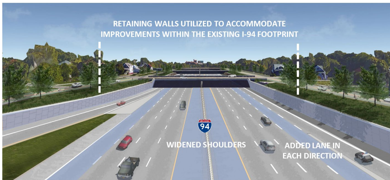
Figure 3-8: Approved Selected Alternative with Modifications Cross-Section
