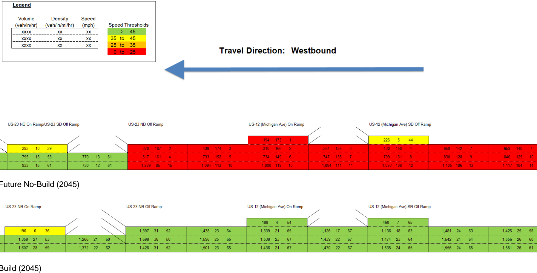
Figure 25: Future No-Build (2045) and Build (2045) Lane Schematic MOE Summary (AM Peak Hour) Example
