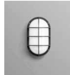
Bega #2841S Tech Wall Luminaire with Poly Diffuser 120V/277V Magnetic Ballast 50 W E-17 HPS Lamp
