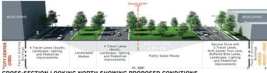
**CROSS-SECTION LOOKING NORTH SHOWING PROPOSED CONDITIONS**
