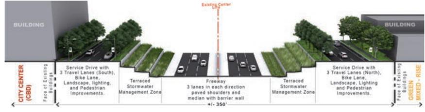
**CROSS-SECTION LOOKING NORTH SHOWING PROPOSED CONDITIONS**
