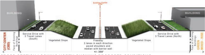
**CROSS-SECTION LOOKING NORTH SHOWING PROPOSED CONDITIONS**
