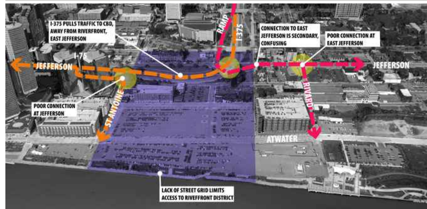
EAST JEFFERSON & I-375 GEOMETRY AND REMOVED STREET GRID LIMIT ACCESS TO RIVERFRONT DISTRICT
