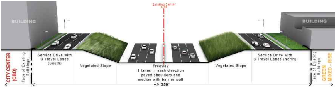
CROSS-SECTION LOOKING NORTH SHOWING PROPOSED CONDITIONS
