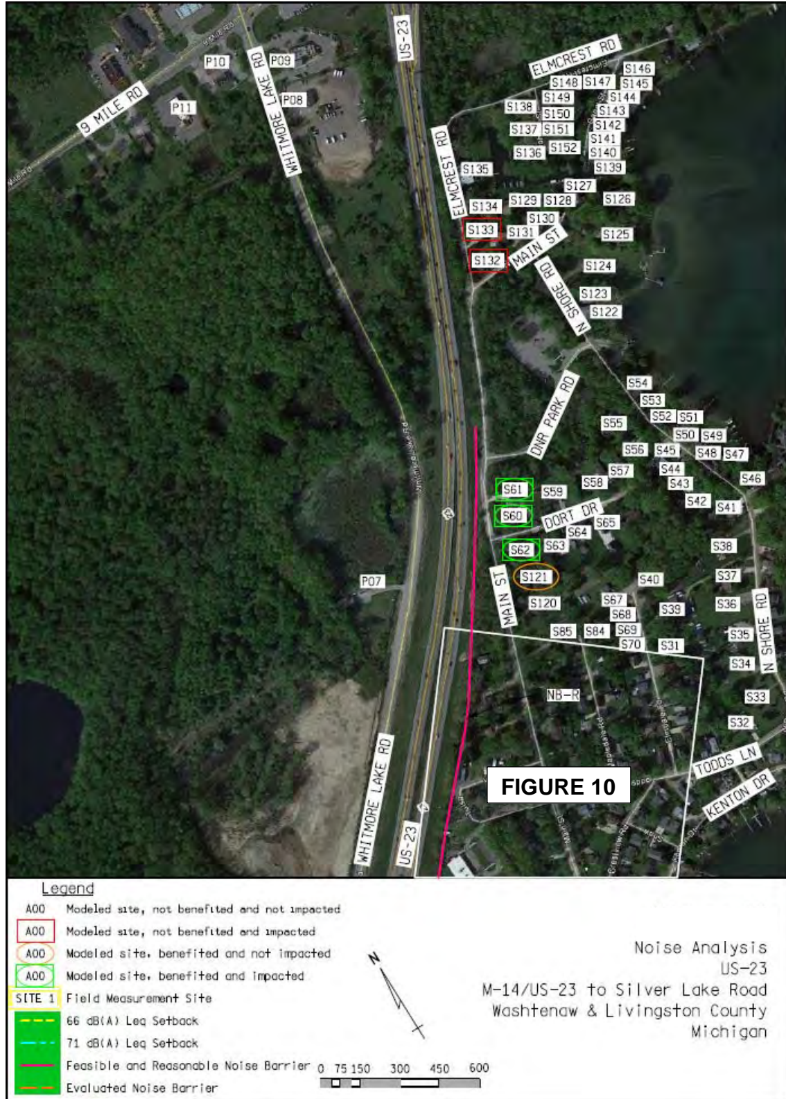
Figure 8: Revised Recommended Barrier – NB-R (North End)
