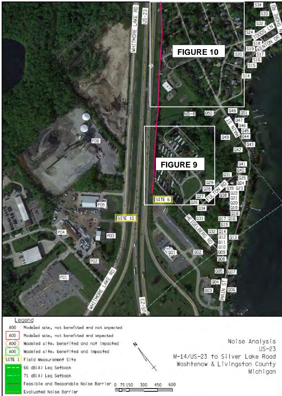
Figure 7: Revised Recommended Barrier – NB-R (South End)
