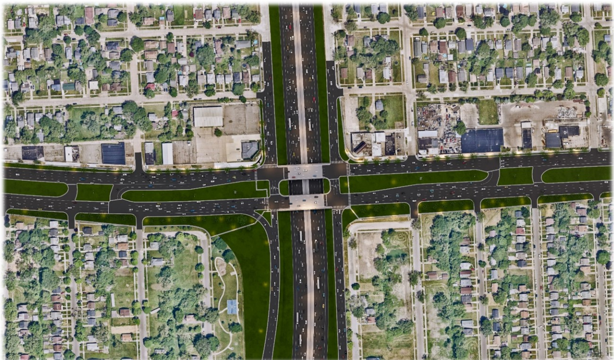
Figure 1. Recommended Concept - Urban Diamond Interchange Layout
