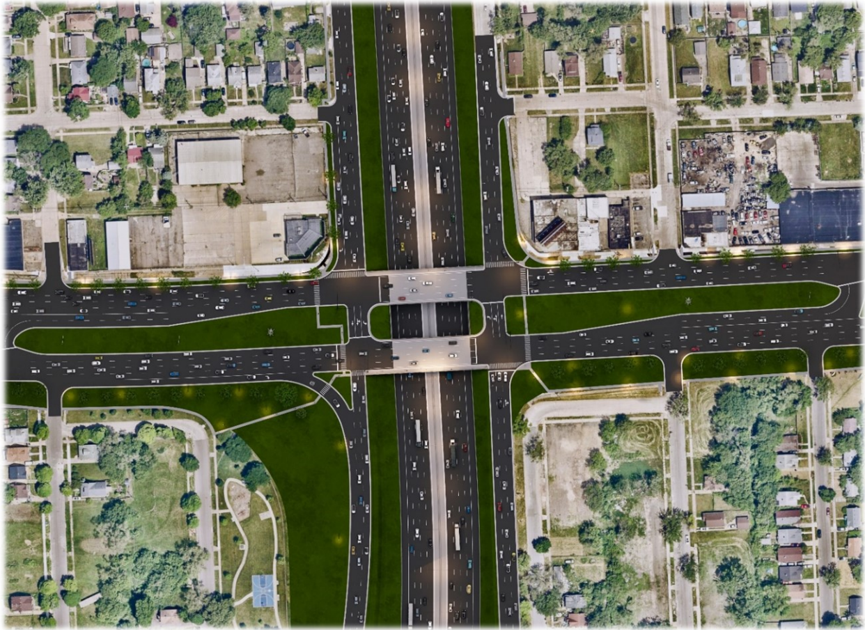
Figure 12. Recommended Urban Diamond Interchange Configuration - Streetview
