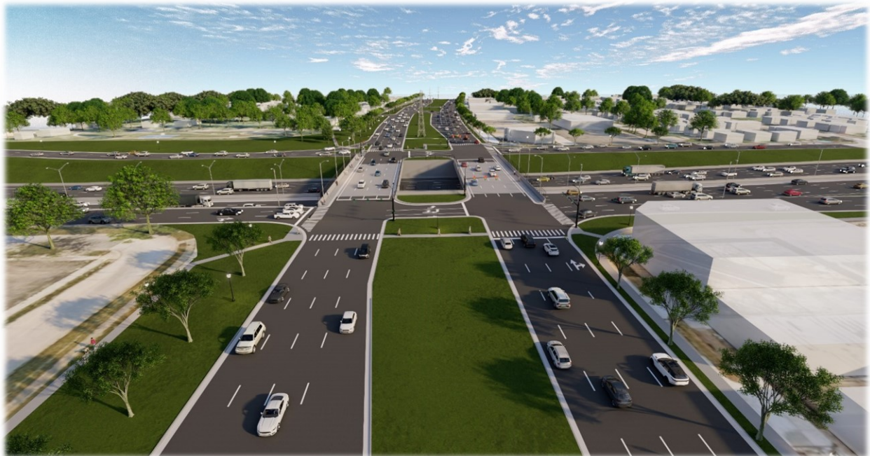
Figure 12. Recommended Urban Diamond Interchange Configuration - Streetview
