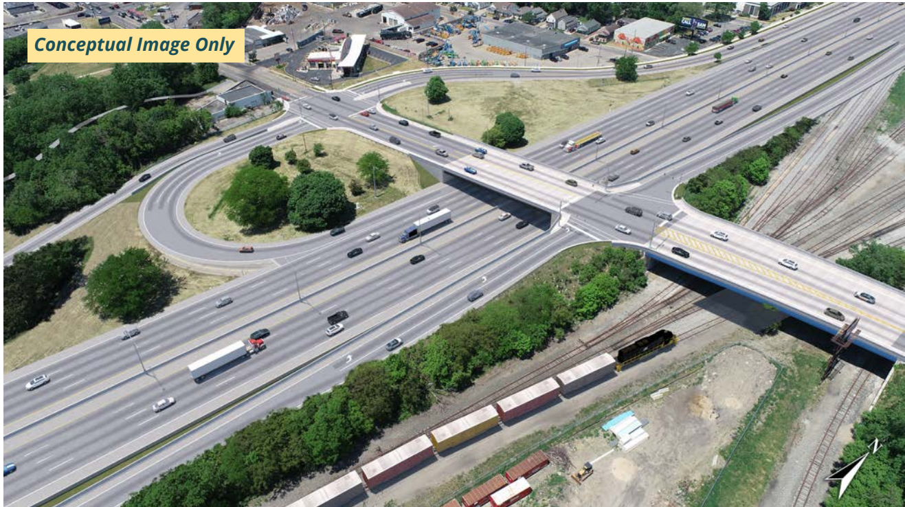
FIGURE 5-8. Burton Street Interchange: Combined Southbound Off Ramps
