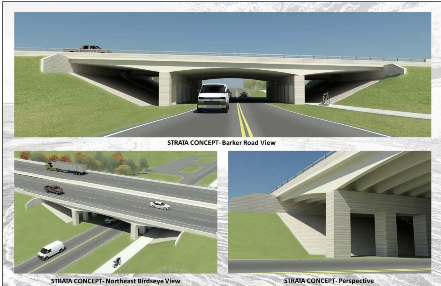
FIGURE 23 – BARKER ROAD STRUCTURE – CONCEPT RENDERINGS – GEOMORPHIC STRATA
