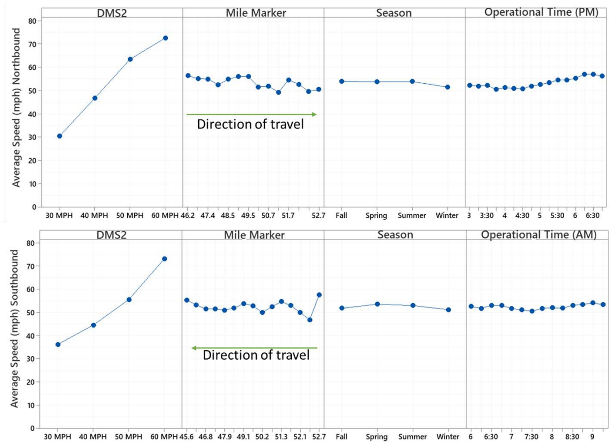
Figure 3-25 Mean speed versus DMS2, mile marker, season, and operational time for both northbound and southbound
