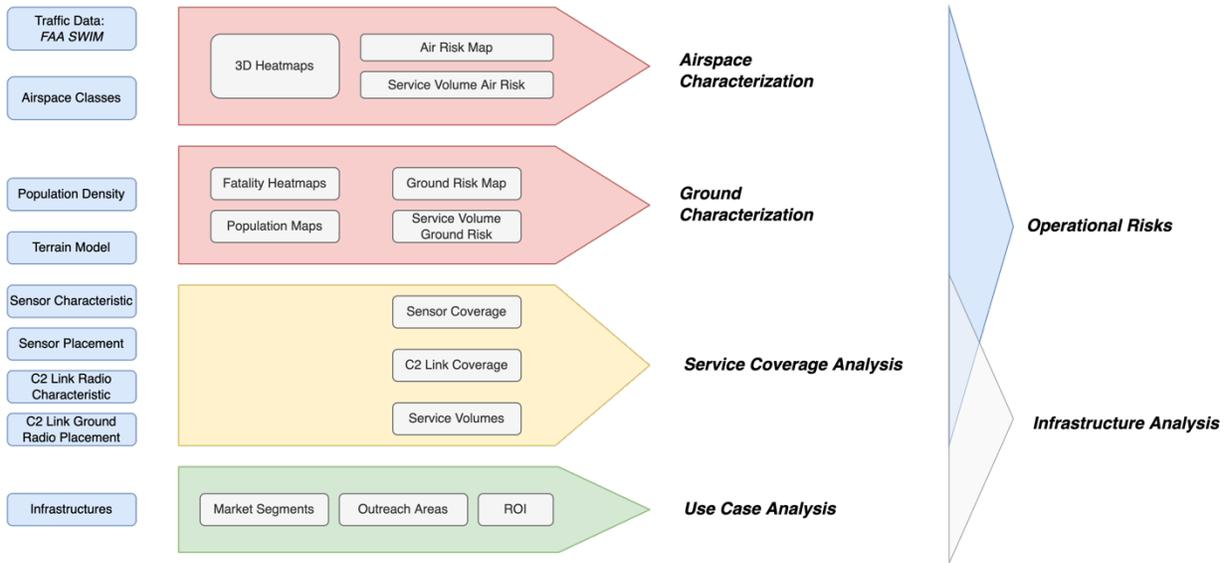
**Figure 9: Airspace Characterization Process as Part of the Overall Operational Risks and Infrastructure Analysis Process**
