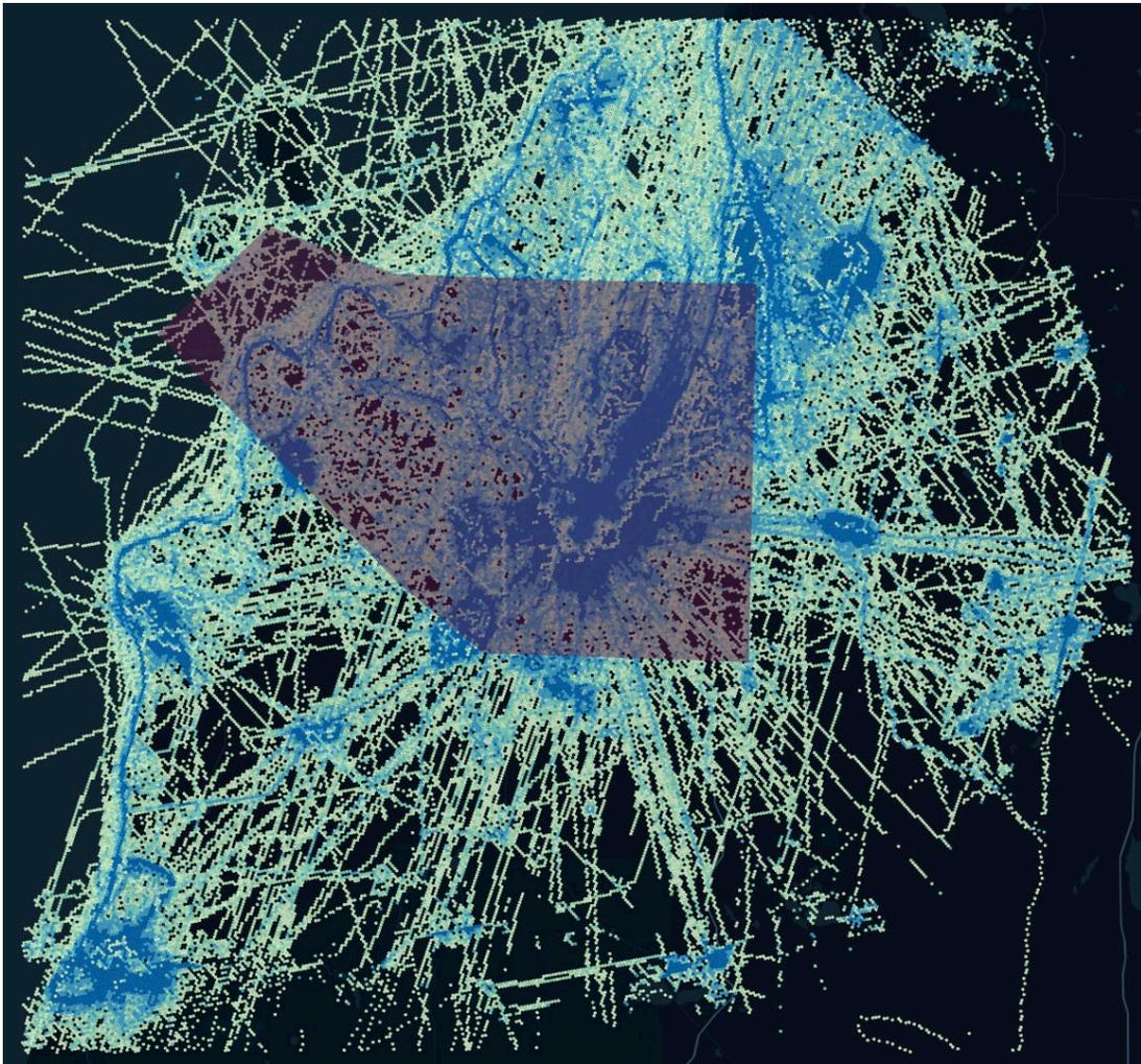
**Figure 50: Example of a UAS Static Air Risk Map with Computed Air Traffic Density <1,200' AGL in Area 3**
