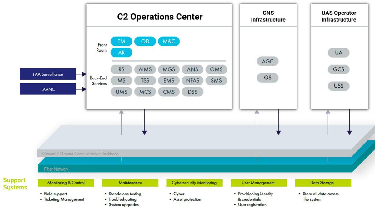
**Figure 79: MDOT BVLOS System Architecture**
