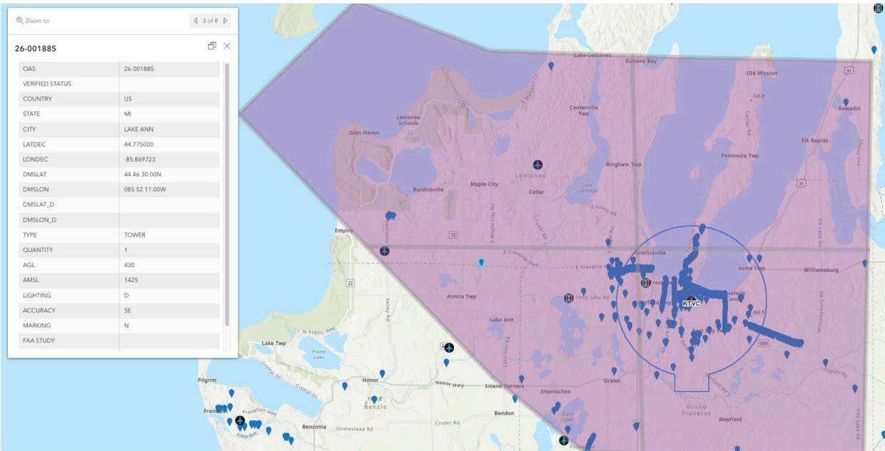
**Figure 49: Obstacles in Area 3 (authoritative source: FAA Digital Obstacle File). A tower is highlighted as an obstacle that stands at 430' AGL.**
