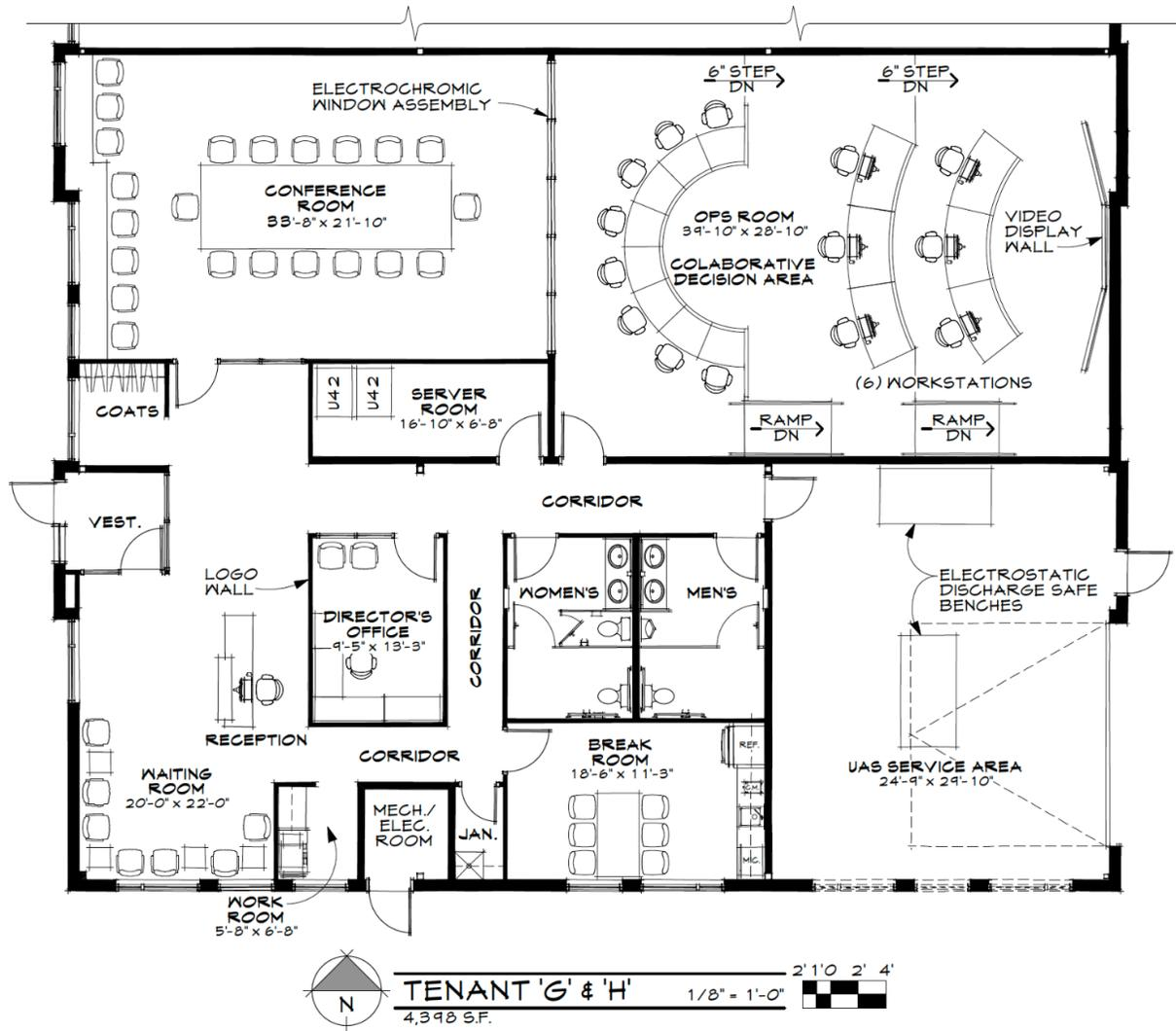
**Figure 80: Example of Floorplan for C2 Center and Space Utilization**
