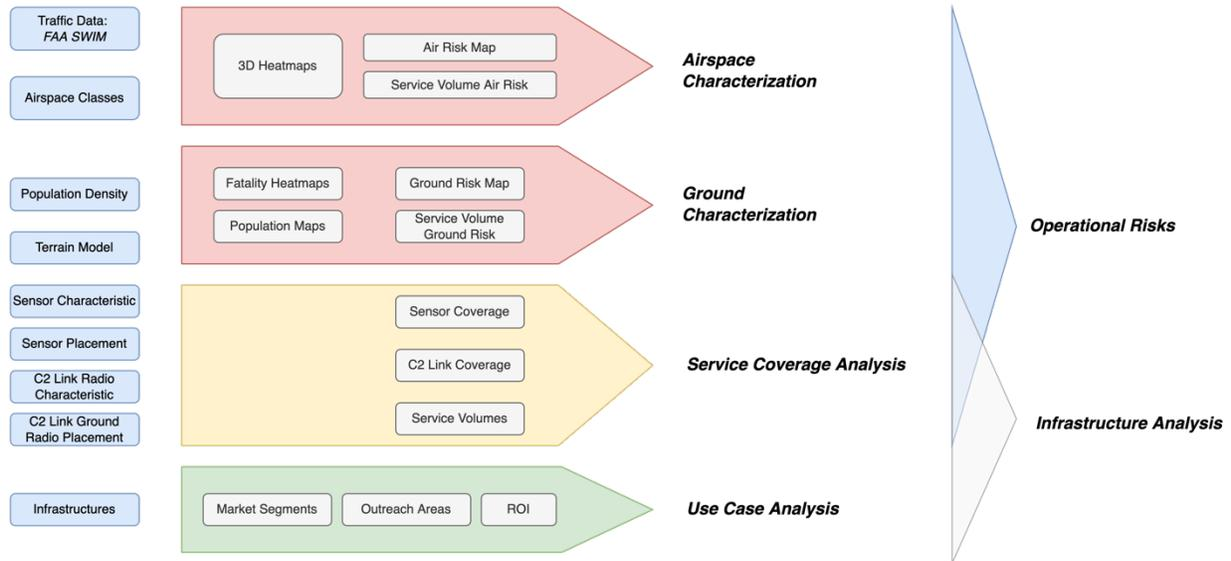
**Figure 41: Airspace Characterization Process as part of the Overall Operational Risks and Infrastructure Analysis Process**
