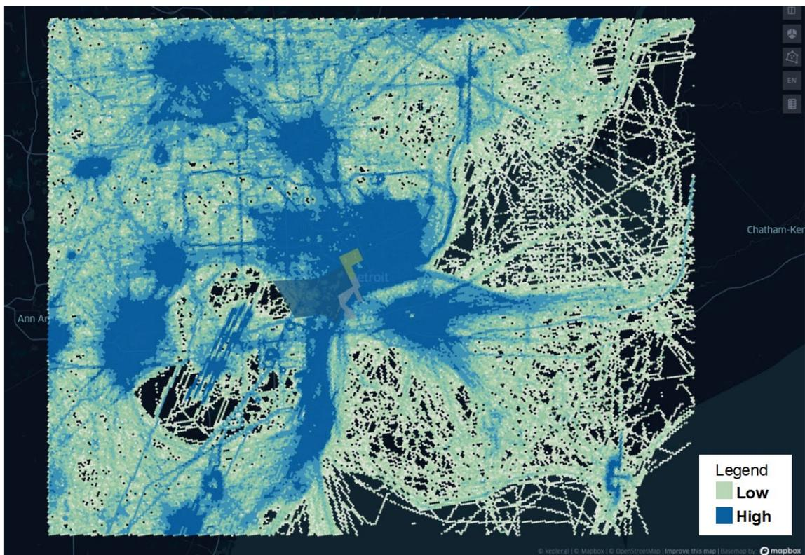
**Figure 19: Example of a UAS Static Air Risk Map with Computed Air Traffic Density of <1,200' AGL in Areas 1 and 2**
