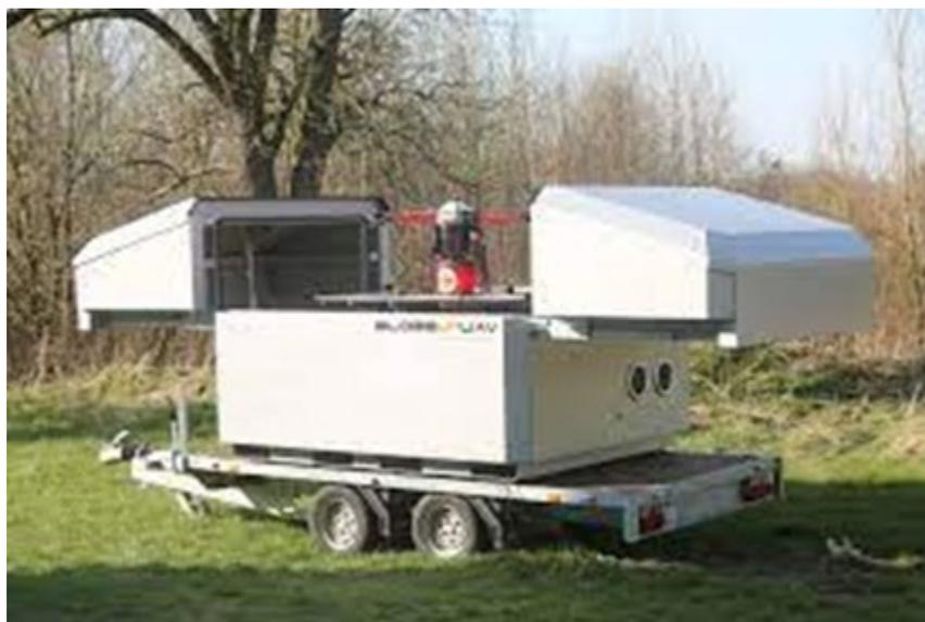
**Figure 74: Drone Docking Station Mounted on a Portable Trailer**
