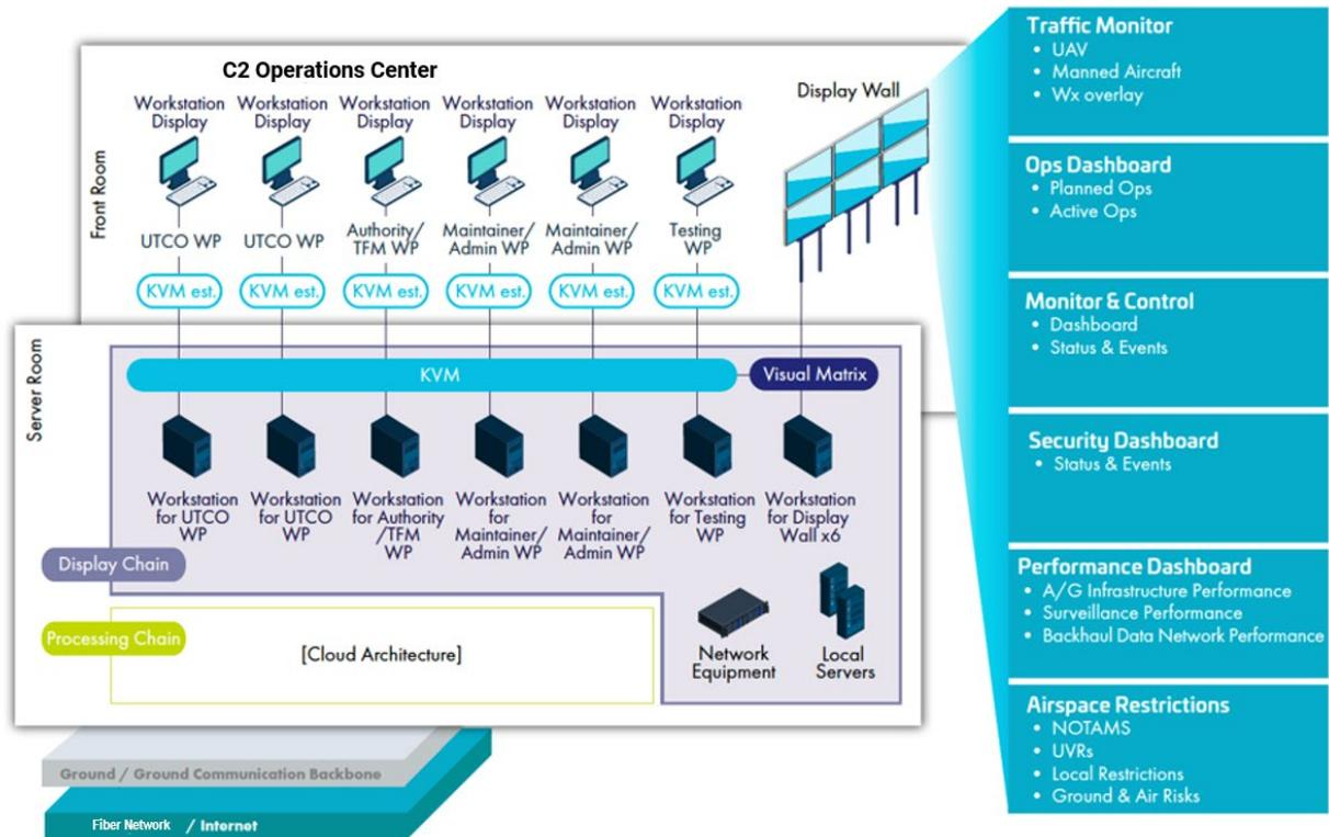
Figure 81: Example C2 Workstation Networking
