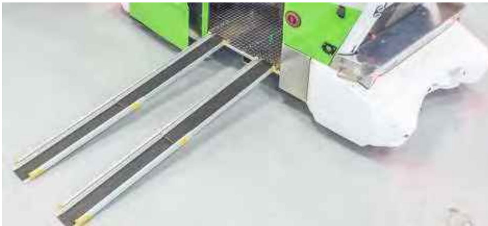
First modified shuttle – “two track” ramp
