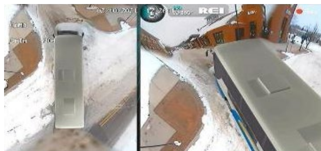
Bay Area Transportation Authority 360-degree detection system
