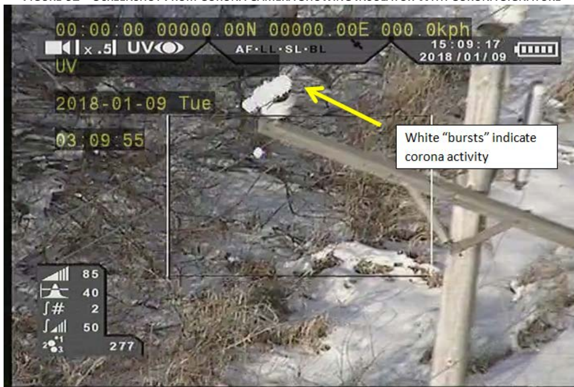
FIGURE 62 – SCREENSHOT FROM CORONA CAMERA SHOWING INSULATOR WITH CORONA SIGNATURE
