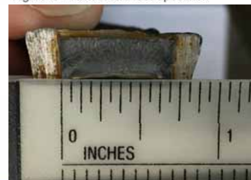
Figure 5—Nick-break Test Specimen
