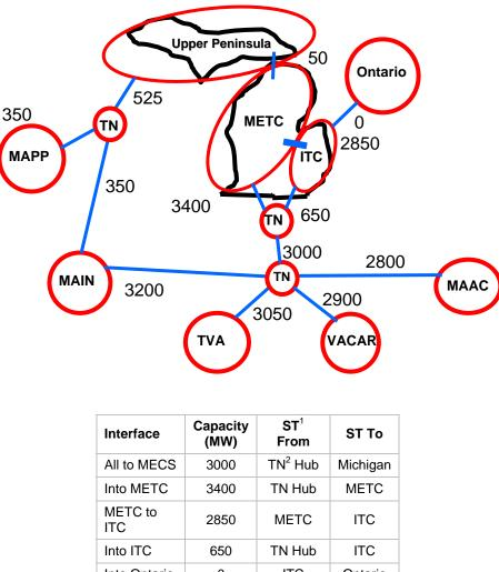
Figure 9: Transmission Interface Capability in 2009 (in MW)
