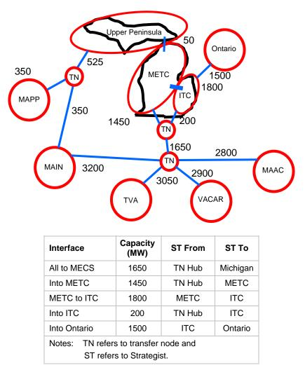
Figure 10: Low Estimate of Transmission Import Capabilities in 2009 (in MW)
