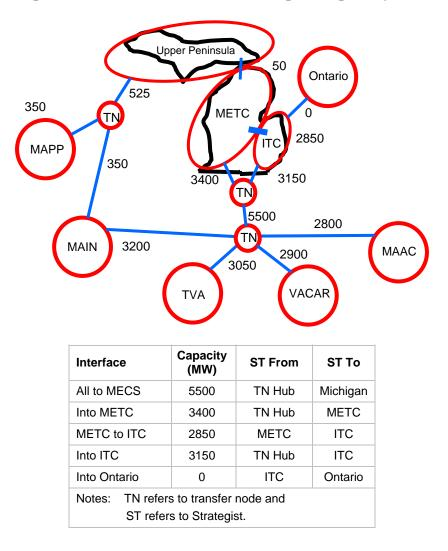
Figure 11: Expanded Estimate of Transmission Import Capability in 2009 (in MW)
