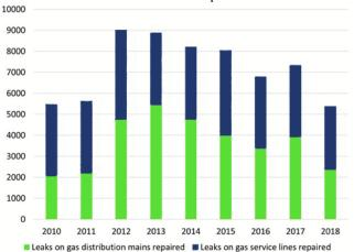
Corrosion-Related Leaks Repaired 2010-2018
