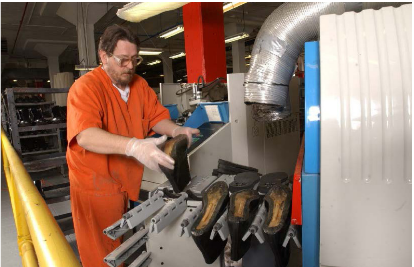
MSI Shoe Shop worker using a heat press machine to mold uppers and soles together
