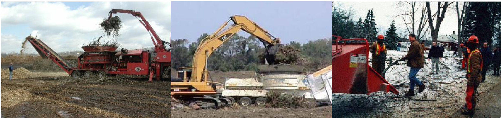
L-R: Tub grinders and brush chipper being loaded with material to be mulched. Tub grinders are suitable for use at TDSR Sites, while brush chippers are more appropriate for smaller sites.
