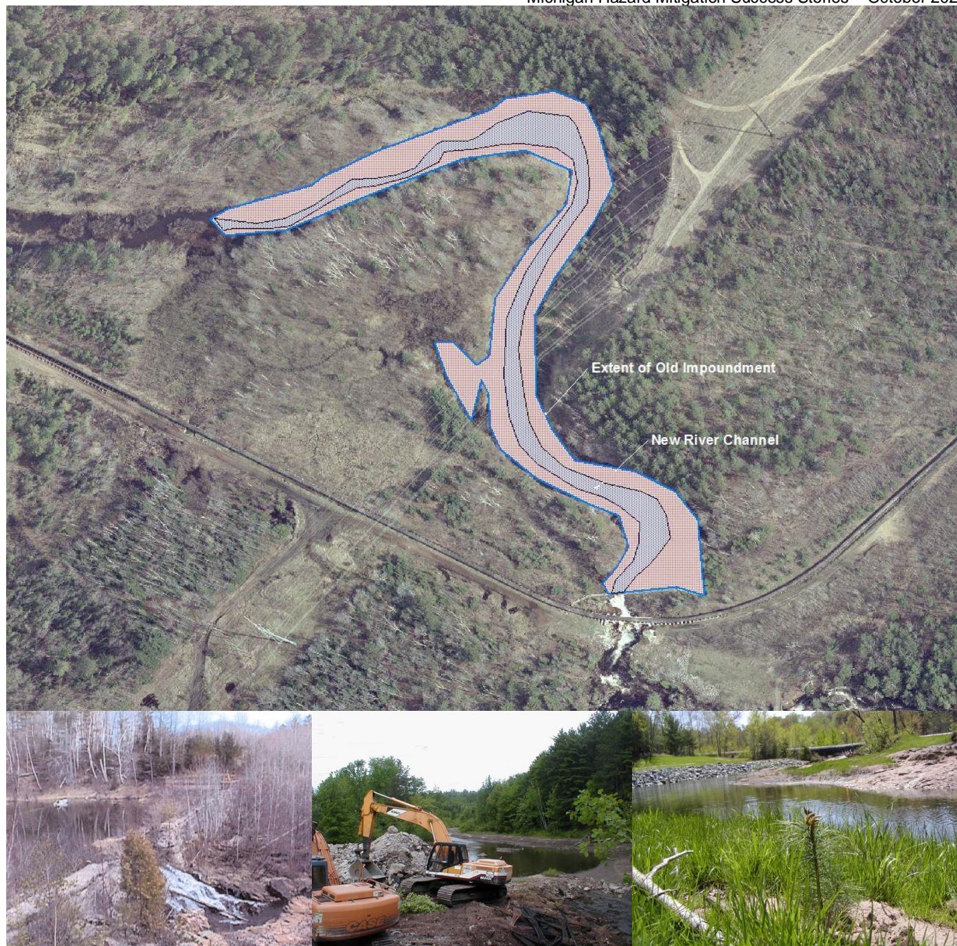
Top Row: Aerial photo depicts the old impoundment and new river channel. Bottom Row L-R: Collinsville Dam before removal; excavators removing the dam; re-vegetation and rip-rap along the river after dam removal.
