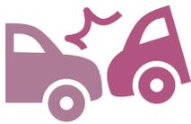
**FORWARD COLLISION WARNING (FCW) AND AUTOMATIC EMERGENCY BRAKING (AEB):** FCW warns the driver of a possible collision with warning lights and sounds. AEB automatically applies the brakes if the driver fails to respond to the warning. [Warning: May encourage teen drivers to tailgate.]
