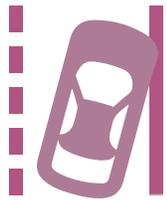
**LANE DEPARTURE WARNING (LDW) AND LANE KEEPING ASSISTANCE (LKA):** LDW alerts the driver with a warning sound, vibration, or visual cue if they drift out of their lane. LKA then automatically steers the driver back into their lane. [Warning: These features may not work if lane lines are faint or covered by snow or debris.]
