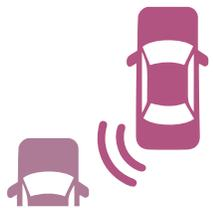
**BLIND SPOT WARNING:** Helps prevent side collisions and increases awareness of surrounding traffic by warning the driver with a symbol, sound or vibration if a vehicle is in their blind spot.
