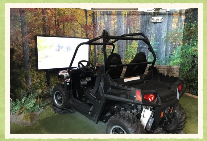
This ATV moves up, down and side-to-side to provide a the feeling of riding on a trail.
