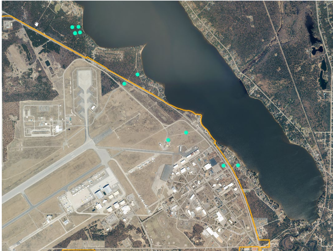
Monitoring Wells Used for Groundwater Flow Determination
