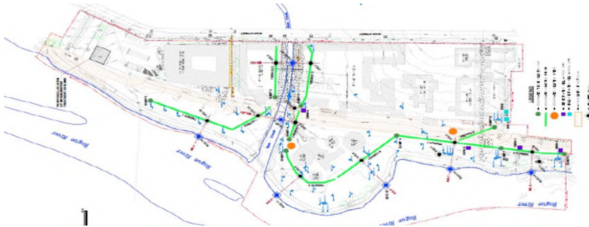
Figure 2. Site Stratigraphy and Proposed Piezometer Arrays for Groundwater Elevation Monitoring
