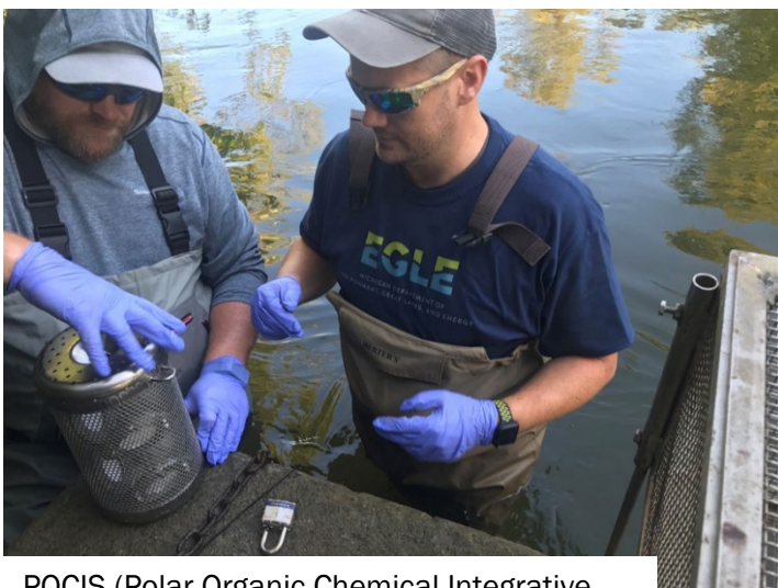
POCIS (Polar Organic Chemical Integrative Samplers) being deployed
