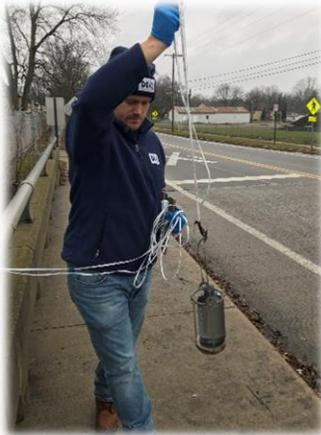
The weighted bottle sampler is typically constructed of a 1-liter Nalgene Tritan® bottle fixed inside a metal cage fitted with a weight below the bottle. This sampler is suspended vertically, which is ideal for sample collection at road or bridge crossings. The bottle is typically lowered to approximately 6-inches below the water surface. The sampler can also be fitted with a depth-integrating cap to allow the bottle to slowly fill while lowering the apparatus to the bottom of the water body.
