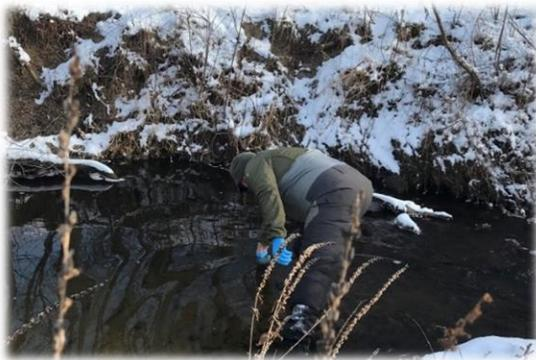
For surface water samples collected near the shore, the direct method can be used to collect the water samples directly into the sample container.
