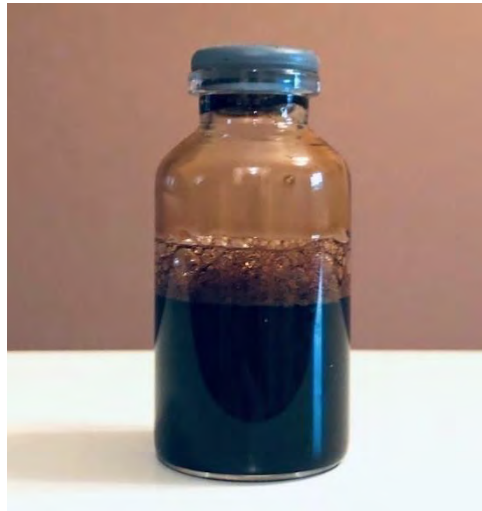
Minute-stable foam derived from agitation of distilled water and humic acid from Leonardite mineral in a 20-ml reaction vessel.
