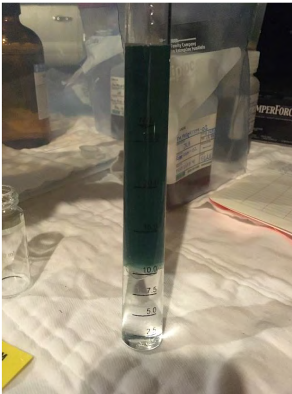
Rogue River SWF sample combined with MBAS suspended on top of chloroform reagent. [11/5/19]
