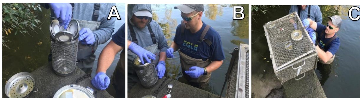
Figure 1. Polar Organic Contaminant Integrative Samplers (POCIS). A: Each POCIS consisted of an Oasis® HLB sorbent sandwiched between two polyethersulfone membranes and two stainless steel rings. B: Six POCIS were deployed at each location and housed in a stainless-steel canister. C: POCIS canisters were secured inside stainless-steel fish cages to stabilize them in the stream and locked to trees along the streambank to prevent theft.
