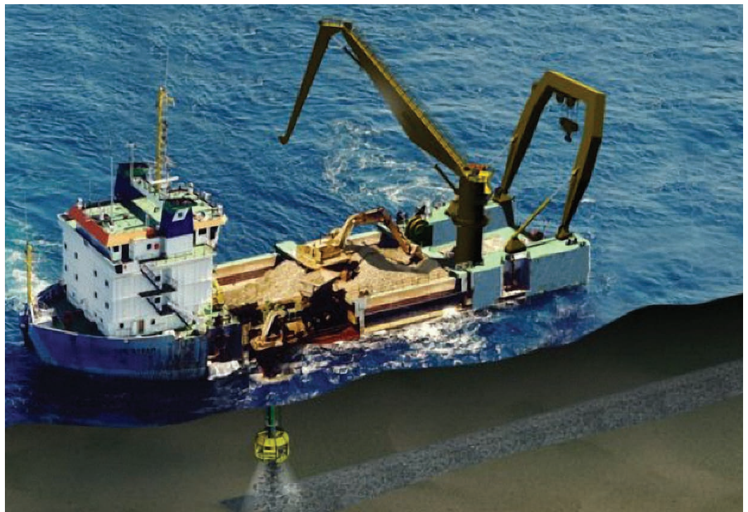
Figure 31: This purpose-built rock placement vessel deploys stone through a side-fall pipe at a controlled rate, while the vessel moves along the pipeline route forming a stone berm to protect the pipeline. The end of the side-fall pipe is controlled from the surface. To provide precision rock placement, the operator uses visual and sonar confirmation of the fall-pipe location relative to the pipeline to be covered.
