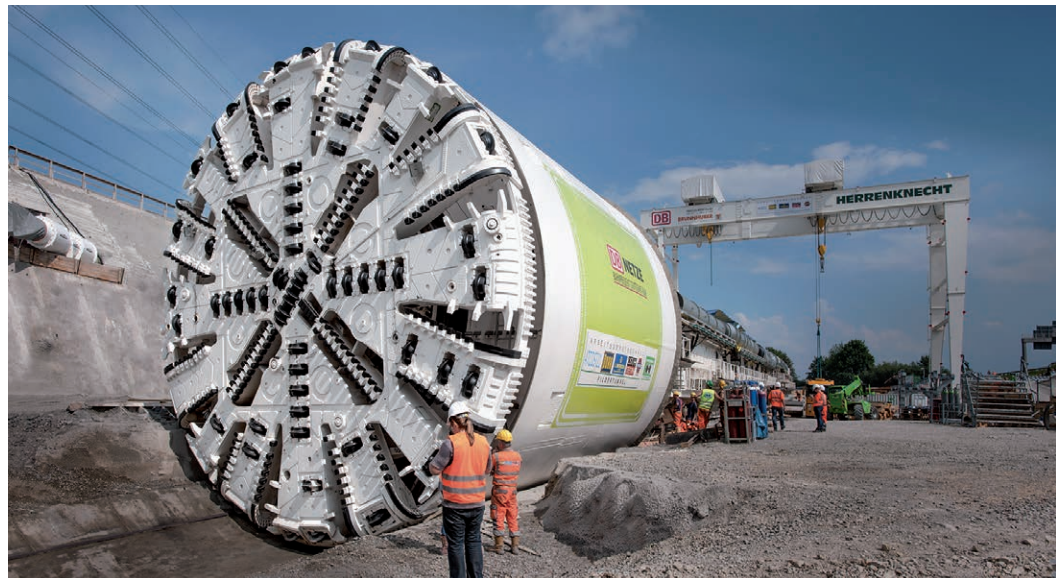
Figure 4: A large TBM—with a 36-foot-diameter cutterhead and shield (foreground) and trailing gear (background) for a total length of almost 400 feet and weight of over 2,200 tons—is readied for the start of construction of the Filder Rail Tunnel in Germany. (Source: Herrenknecht)
