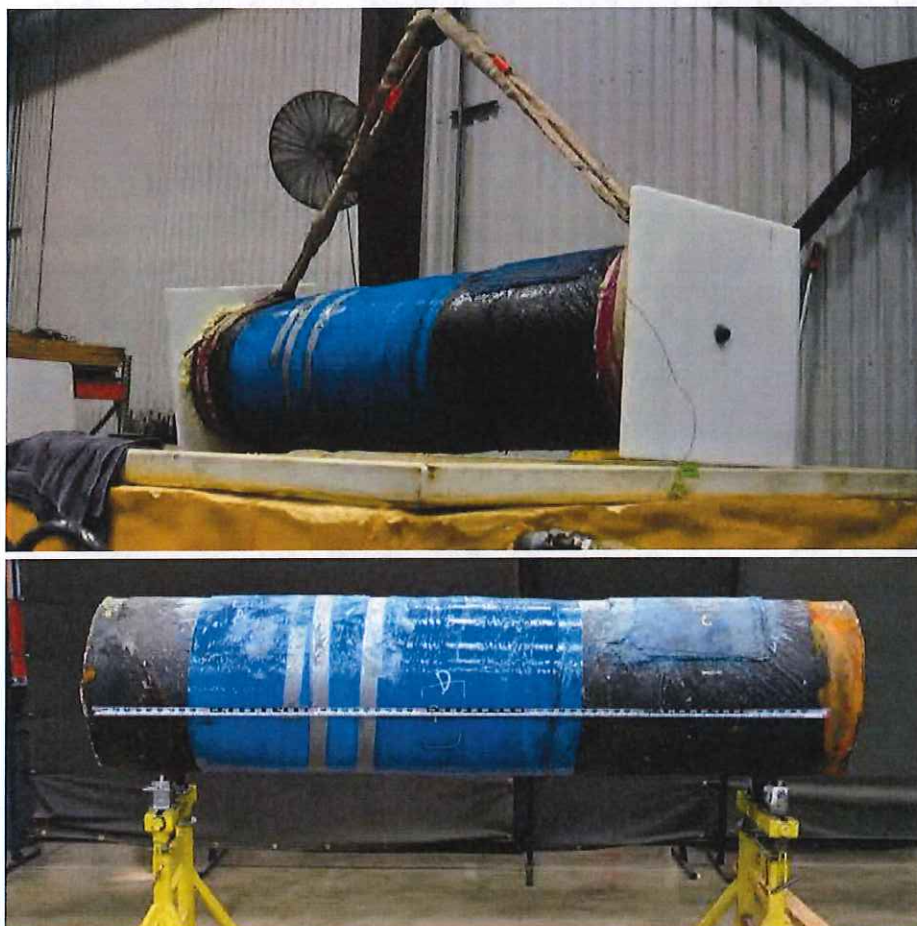
Figure 17: (a) Photograph of 20" pipe sample after removal from water bath; (b) photograph showing stricture still applied to Areas "A" and "B/D/E." Area "C" (patch repair with no stricture) is on right end. Numbered scale divisions are 0.1 feet.
