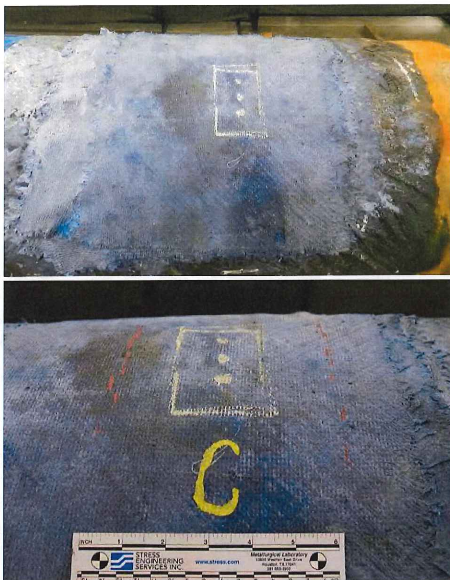
Figure 19: Photographs showing patch repair at Area "C" where no stricture was applied.
