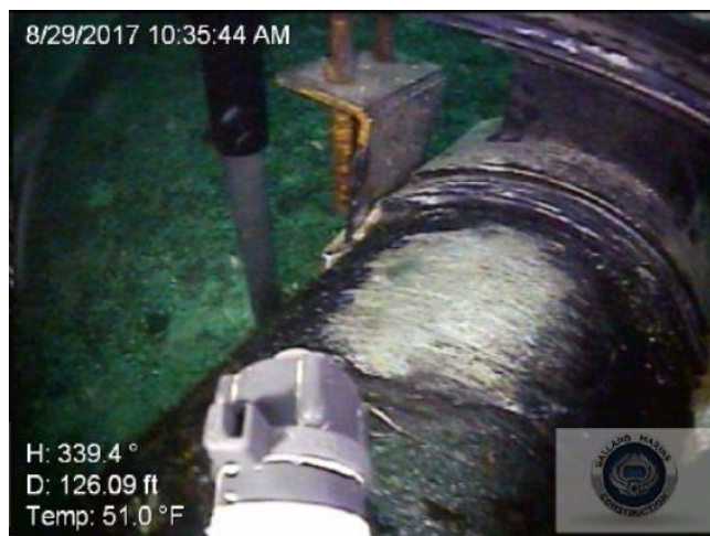
Figure A4: Coating damage found during a pipeline inspection
