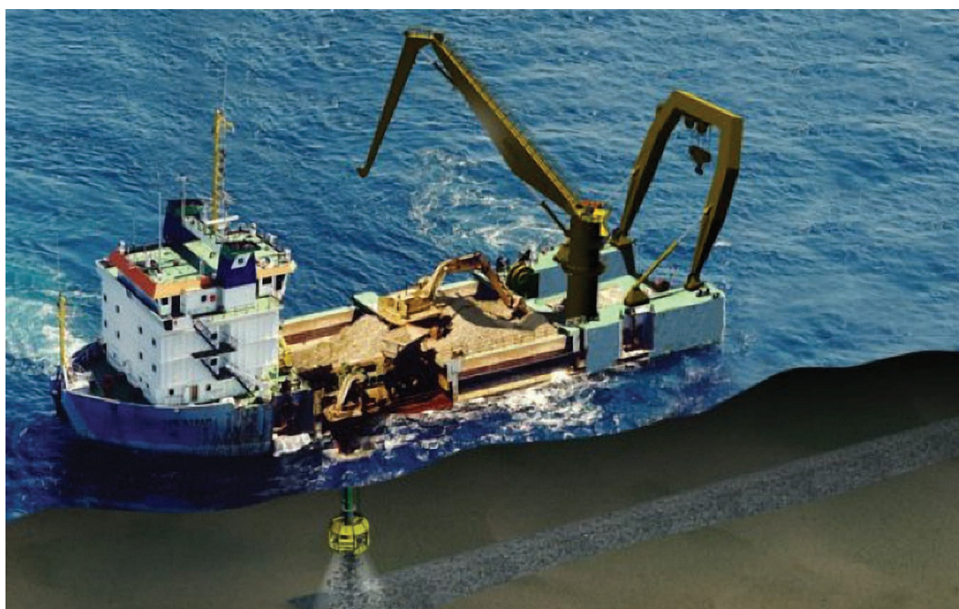
Figure 16: This purpose-built gravel/rock placement vessel deploys the stone through a side-fall pipe at a controlled rate, while the vessel moves along the pipeline route forming a stone berm to cover the pipeline. The end of the side-fall pipe is controlled from the surface. To provide precision rock placement, the operator uses visual and sonar confirmation of the side-fall pipe location relative to the pipeline to be covered.
