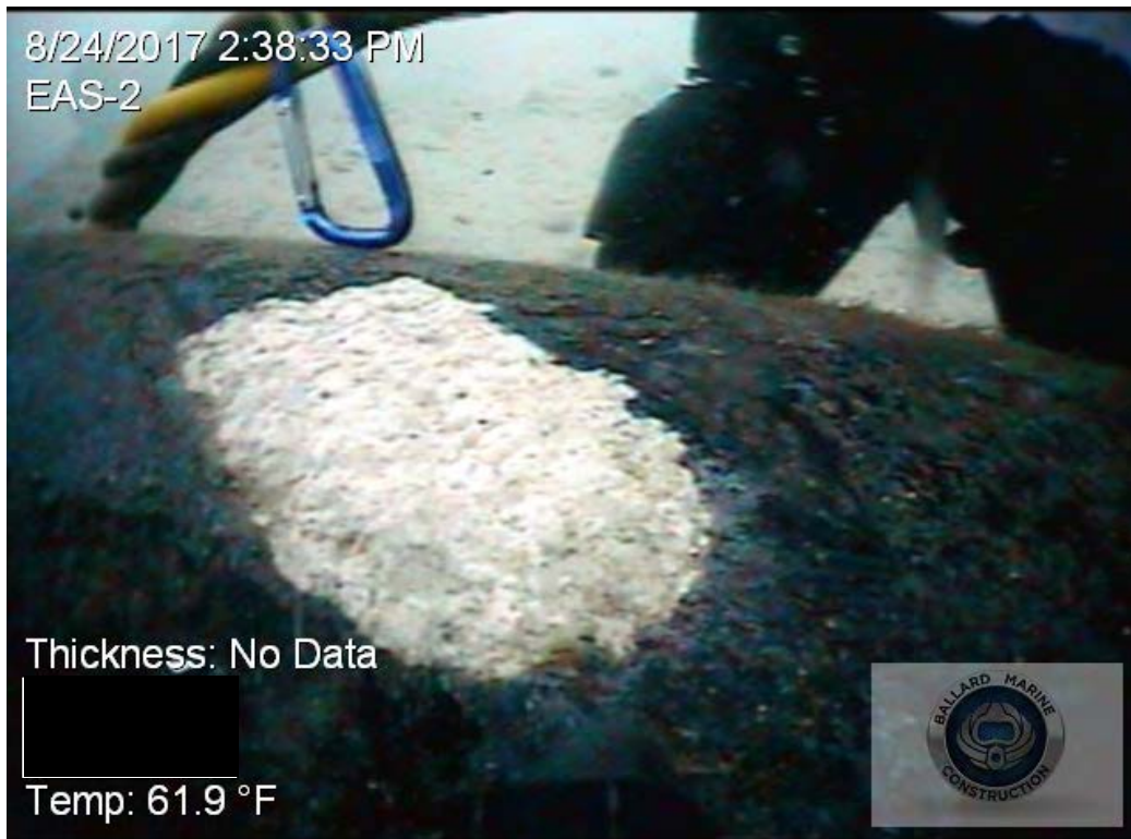
Figure 1: Photograph showing a calcareous deposit at EAS-2
