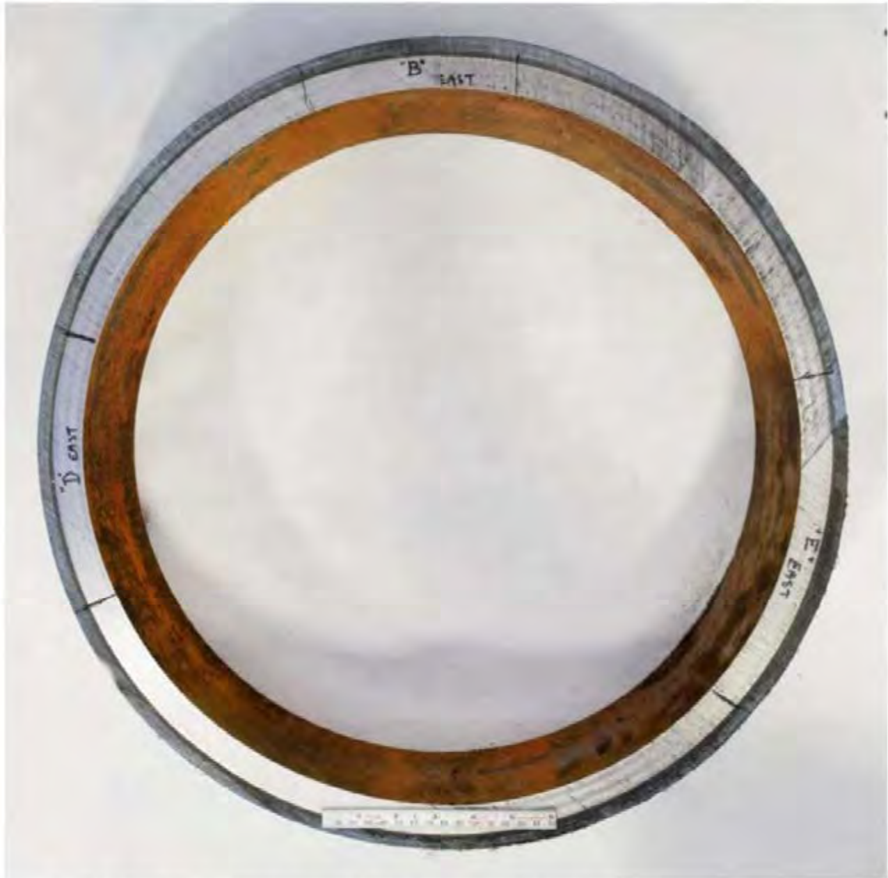
Figure 22: Photograph of cross-sectional ring cut from center of 20" pipe sample containing repair Areas "B/D/E."
