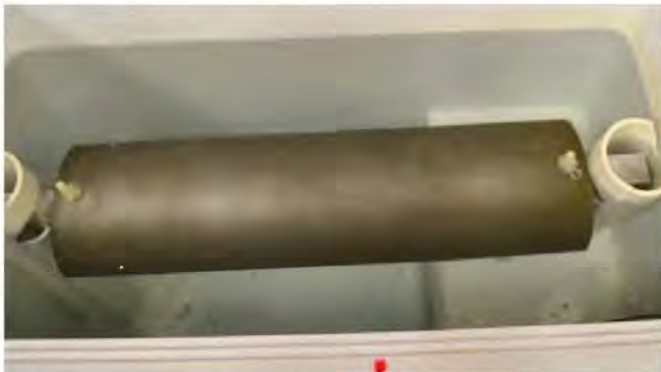
Figure 4: One of two laboratory test samples used for initial tests of repair material. A 6" pipe section is shown submerged in 40°F water prior to application of repair coating.
