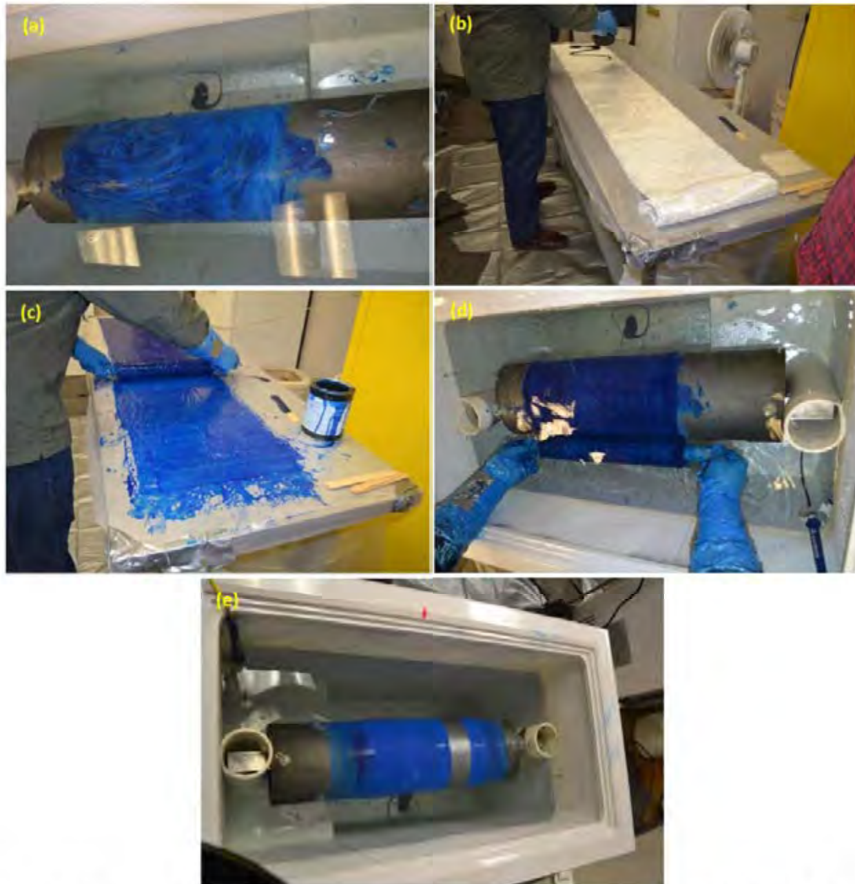
Figure 6: Photographs showing application of laboratory epoxy repair wrap: (a) epoxy applied to bare steel; (b) and (c) fabric impregnated with two-part epoxy; (d) fiber mesh repair wrapped around pipe in four layers; and (e) stricture banding applied over repair.
