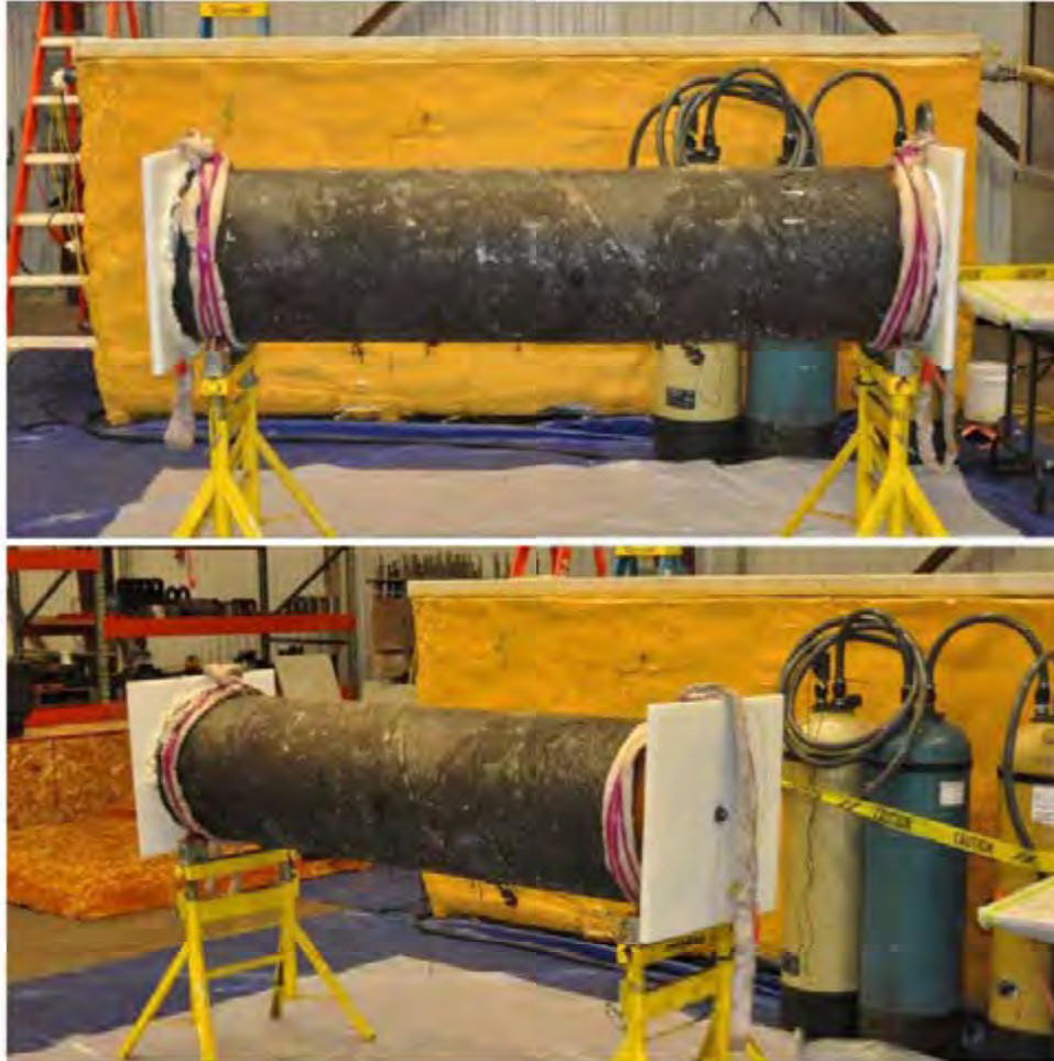
Figure 8: Photographs showing 20" diameter pipe used for full-scale testing of epoxy repair material. Note insulated yellow water tank shown in background.
