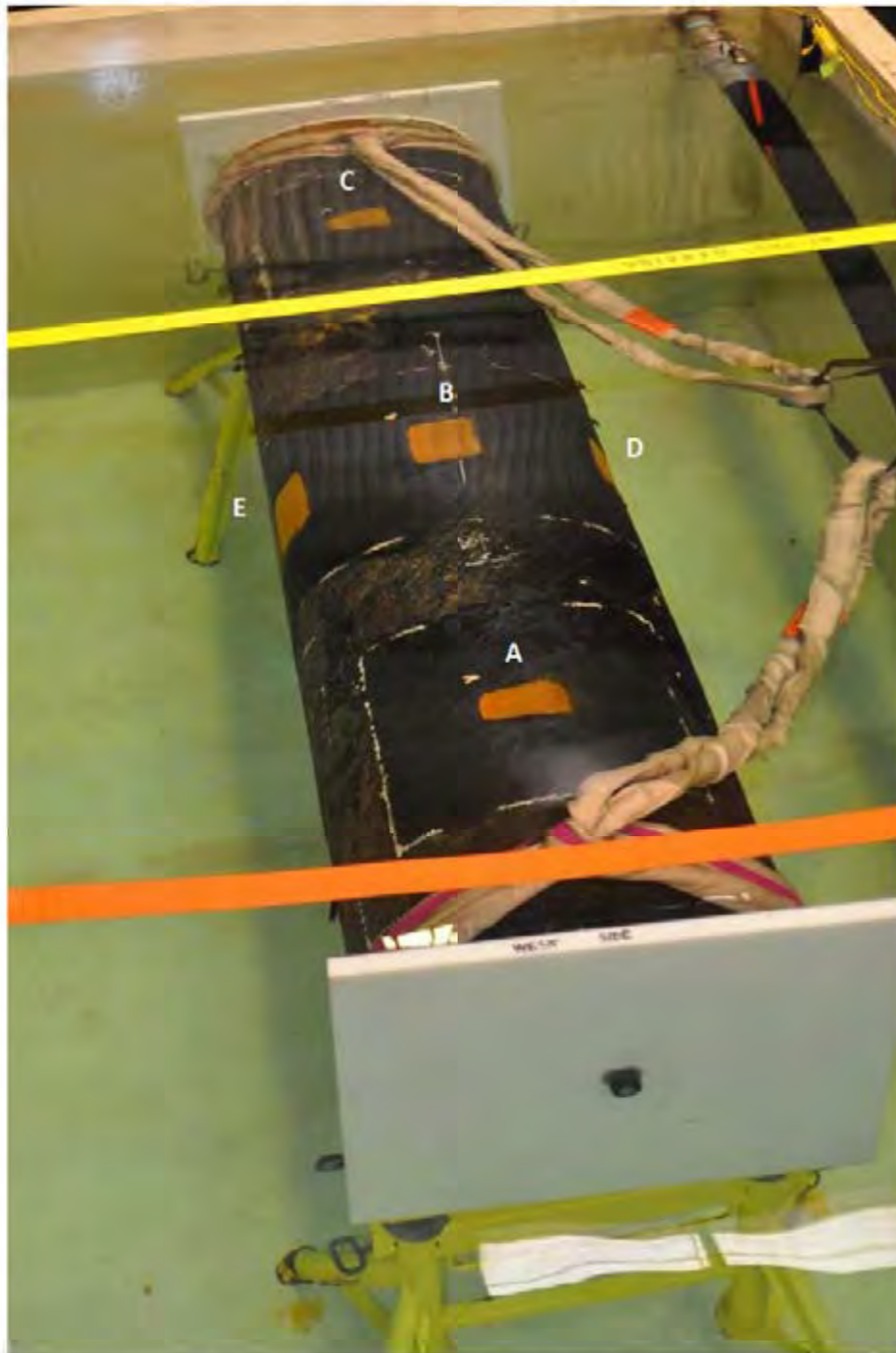
Figure 11: Photograph showing 20" pipe in 40°F water prior to application of epoxy repairs. Repair areas are labeled per Table 1 and Figure 10. Flash rust on exposed areas was removed prior to repair.
