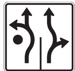
*Signage used at multi lane roundabouts. Use left lane for turning left or going straight. Use right lane for going straight or turning right. Photo courtesy of MUTCD, 2009 Edition, published by FHWA at <https://mutcd.fhwa.dot.gov>.*
